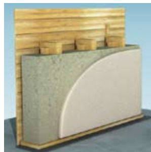
Banchage mur ossature bois
